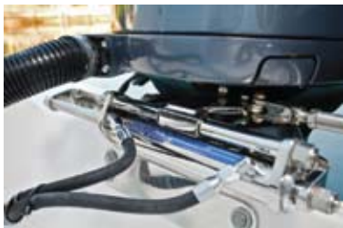
TIGHT GRIP. Latham's side-mount steering system at work on an Intrepid 370 (top). The unit grips a Yamaha F350 outboard (above).
